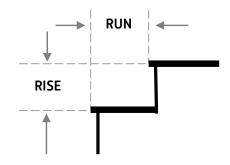
Measure the rise and tread run as shown and use the table to determine the pitch in degrees.
